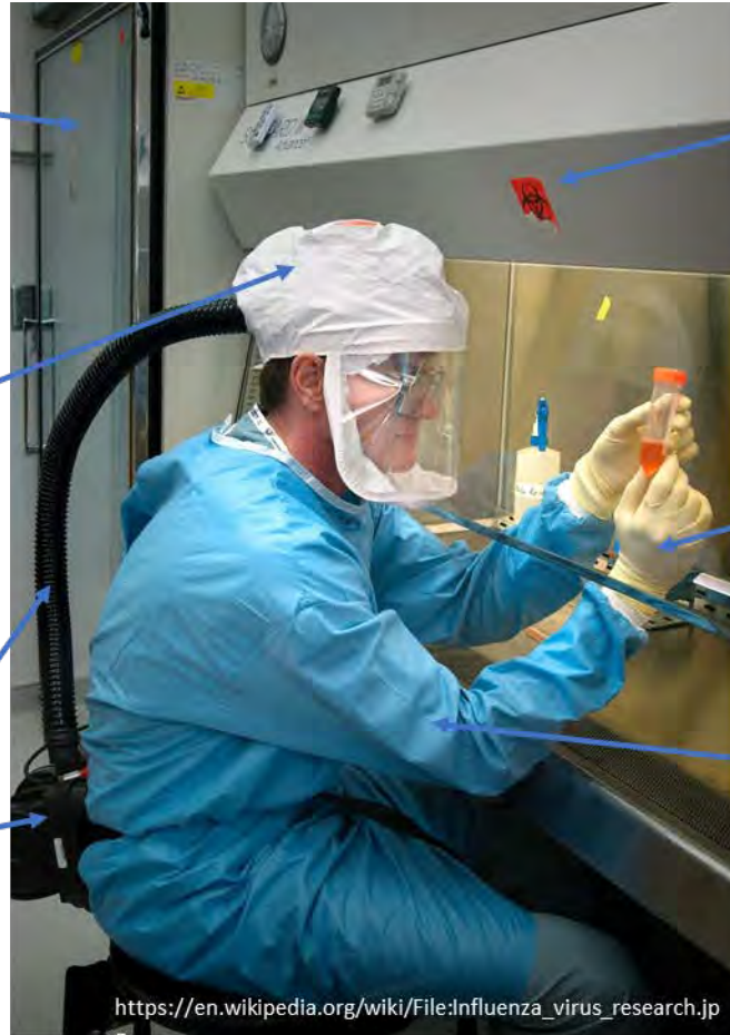
Figure 7: Personal protective equipment required to safely work with containment level-3 pathogens such as SARS-CoV-2.
