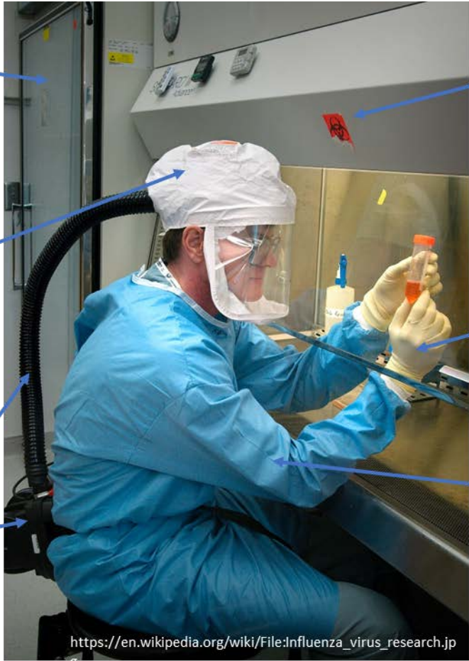
Figure 12 : Personal protective equipment required to safely work with containment level-3 pathogens such as SARS-CoV-2.
